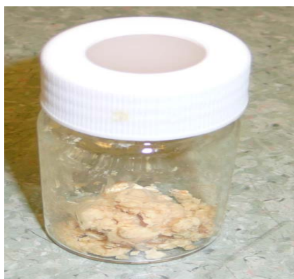
Figure 3: PETE and LDPE waste plastic to fuel production period wax collected from condensation unit
